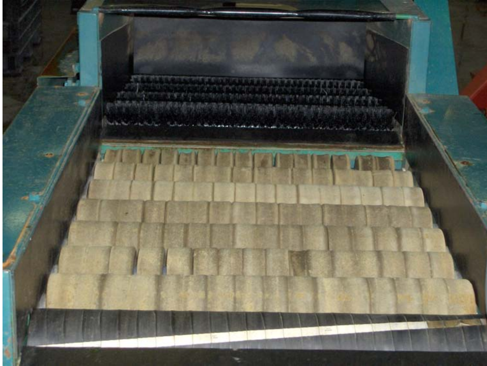
Figure 18: Fruits are automatically dried with soft roller brushes
