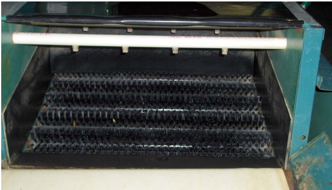
Figure 17: Padded roller brushes are intermittently moistened with sanitizer
